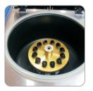
Vacuum port is on the center of rotor to make contamination to be minimized.
