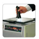
Real scope(option) It is invented to check the remaining amount of sample simultaneously with operation without stopping concentrator.
