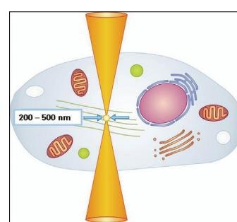
Left: Linear absorption – constant absorption coefficient ( $\mu_a$ ); non linear absorption -  $\mu_a$  depends on intensity of light (fs-laser pulses) and enables a very small focal volume (< 1μm in diameter).
